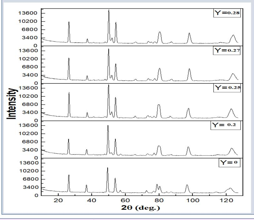
Neutron diffraction patterns of all the selected samples collected at 4.2K are given in Fig. 1. The diffraction patterns contain the magnetic reflections originated only the Mn moments contribute to the magnetic neutron scattering.
